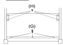
3. Fasten (A) and (B) with four screws (H) from the front and fasten (B) and (C) with three screws (G) from the back.
